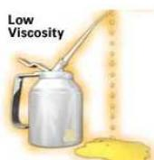
**V**iscosity is a measure of the fluid's resistance to flow. Water has a low viscosity of 1 cSt and honey has a very high viscosity, lets say 1,000 cSt.
